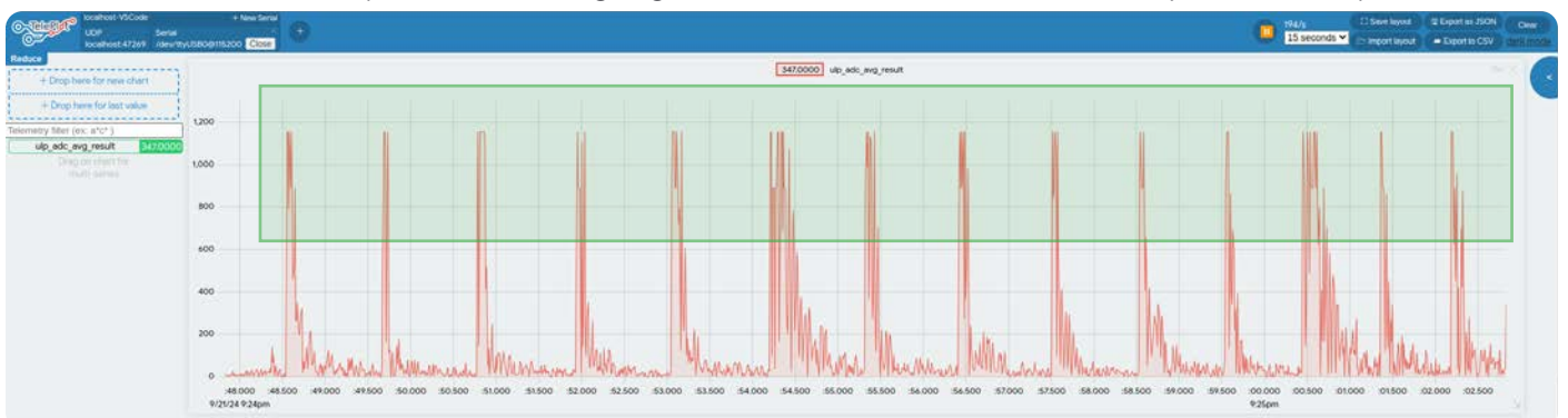
The onboard microphone detecting regular knocks on the door, as read by the ULP coprocessor.
